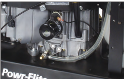
Easy to change oil filter with drain hose.
