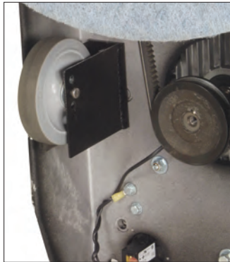
Easy pad pressure adjustment with 4 position wheels.
