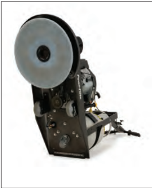
Easy pad change and inspection with tilt up position.
