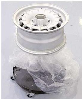
*The easiest way to paint a wheel is to place it on a plastic-covered Pneumatic Sit-On Creeper and gently spin the wheel as you paint.*
