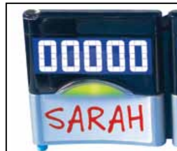
When a player signals to register, her signal light will light up. The numbers 00000 will appear on the scoreboard. This enables you to see that all the LCD segments are functioning.
